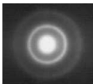
Fig. 2.13: Electron diffraction pattern from nickel crystal
