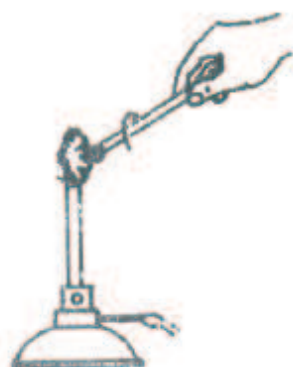
Fig. 2.1: Sealing of Capillary tube
