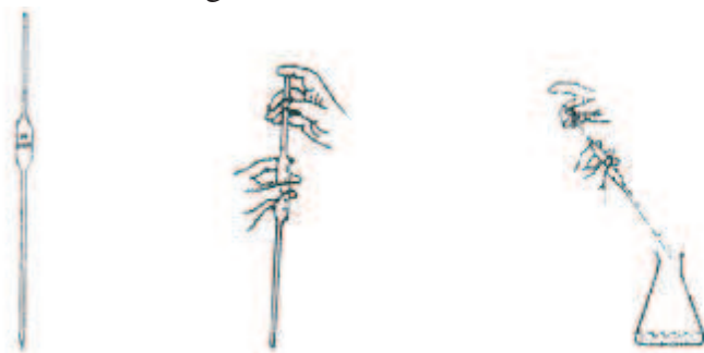
Fig. 15.2 (a): Pipette (b) Handling of a pipette (c) Correct way to drain out the solution
