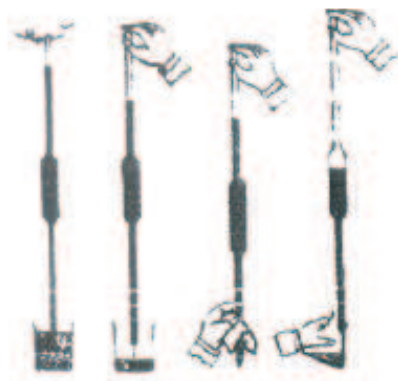
Fig. 15.3: Measuring of solution with a pipette
